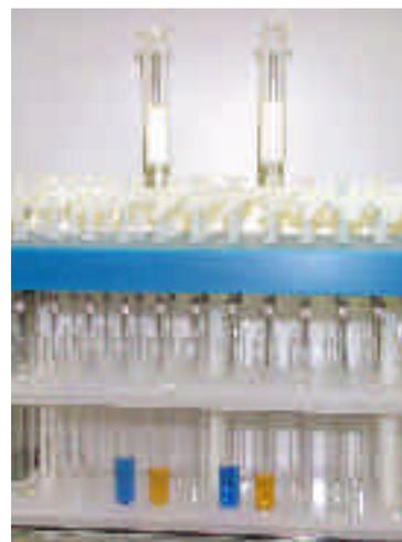
The cartoon shows the separation of an organic (blue) compound from a fluorous (orange) compound by SPE over *FluoroFlash*<sup>™</sup> silica. The photo shows duplicate completed experiments conducted with an organic dye (Solvent Blue) and a fluorous dye (F-Orange-I, C<sub>7</sub>F<sub>15</sub> tag). These aminoanthraquinone dyes have about the same polarity and cannot be separated by regular or reverse phase silica gel. The cartridges can be reused.
